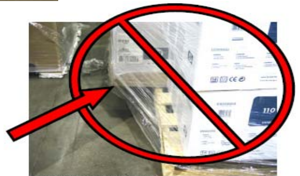
Overhang Configuration Increases the risk of damage to product.
